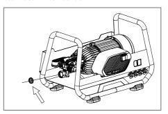
The pressure washer is equipped with a water inlet screen to protect the pump. If the screen is not kept clean, the flow of water to the pressure washer will be restricted, and the pump may become damaged.
