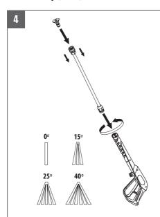
To install tip, gently slide the collar back before inserting it, then release the collar to lock the tip.
