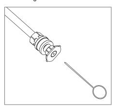
Clogging of the nozzle causes the pump pressure to be too high, making it necessary to clean the nozzle immediately. You can clean the nozzle by carefully inserting the cleaning needle or a thin, sharp instrument (i.e. paperclip) into the tip to clean out any deposits.
